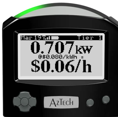
Figure 5-18: Aztech Information Display of Real Time Usage and Cost
