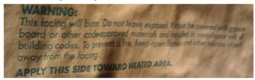
The entire floor of the home inside the crawlspace is covered in this manner. This installation poses a fire danger to the homeowner and this batting should be removed and new insulation should be placed correctly to insulate the floor of this home. Insulation with a non-flammable exposed surface should be installed in spaces where the insulation is exposed as it is with this installation.
