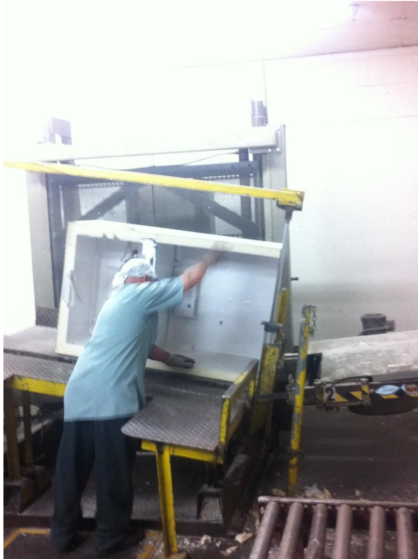
Figure I-6. Segmenting of Unit for Foam Removal (ARCA Compton Facility)
