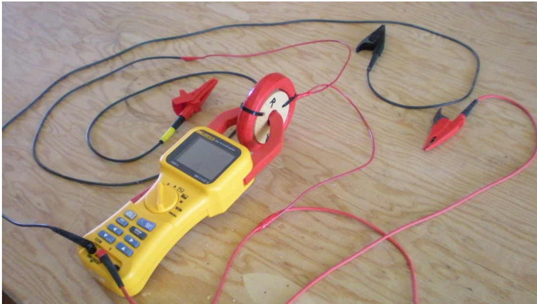
Figure G-6: Standard Setup for the Current Amplifier and Multimeter
