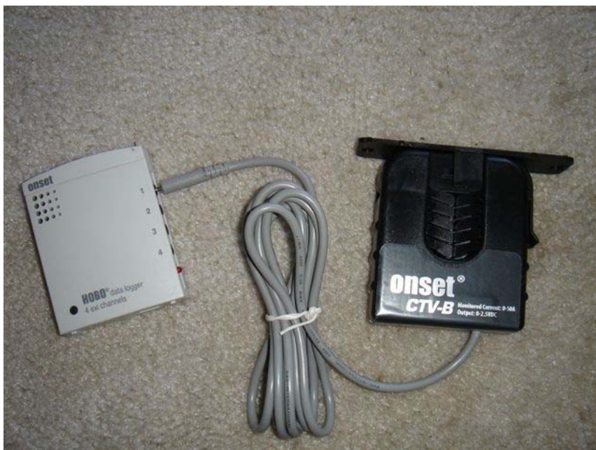
Figure G-4: Onset CTV-A/B/C with Onset HOBO 4-Channel Data Logger
