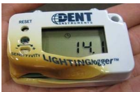
Figure G-7: Example of a Heat-Damaged Logger
