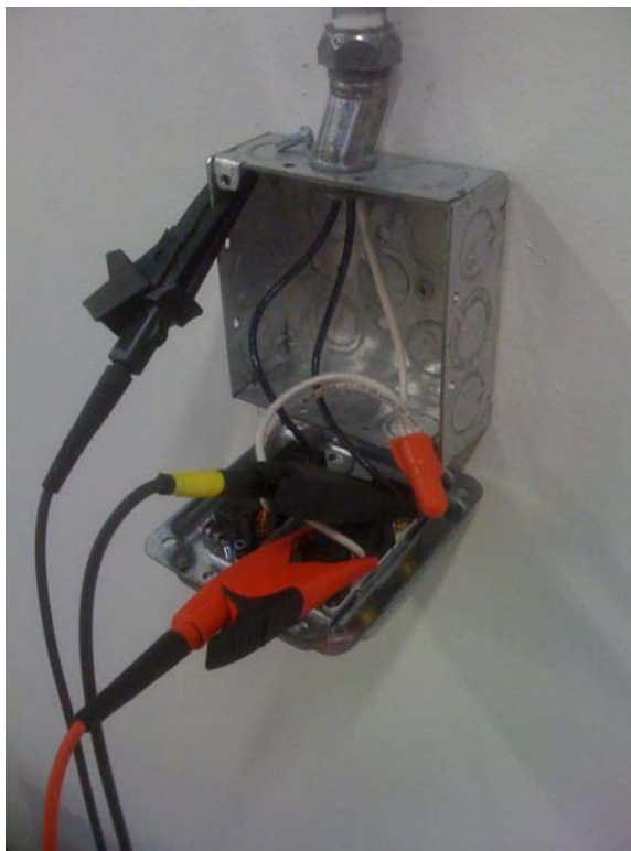
Figure 11. Setup for Switch-Level Measurements with Current Amplifier
