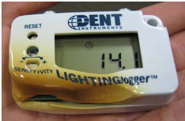
Figure B-10: Melted Lighting Logger
