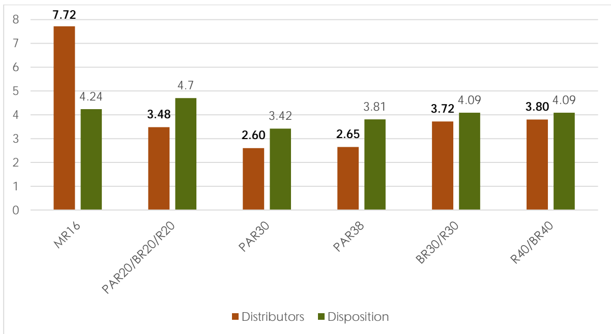
Figure 4-4. Reflector Wattage Reduction Ratios
