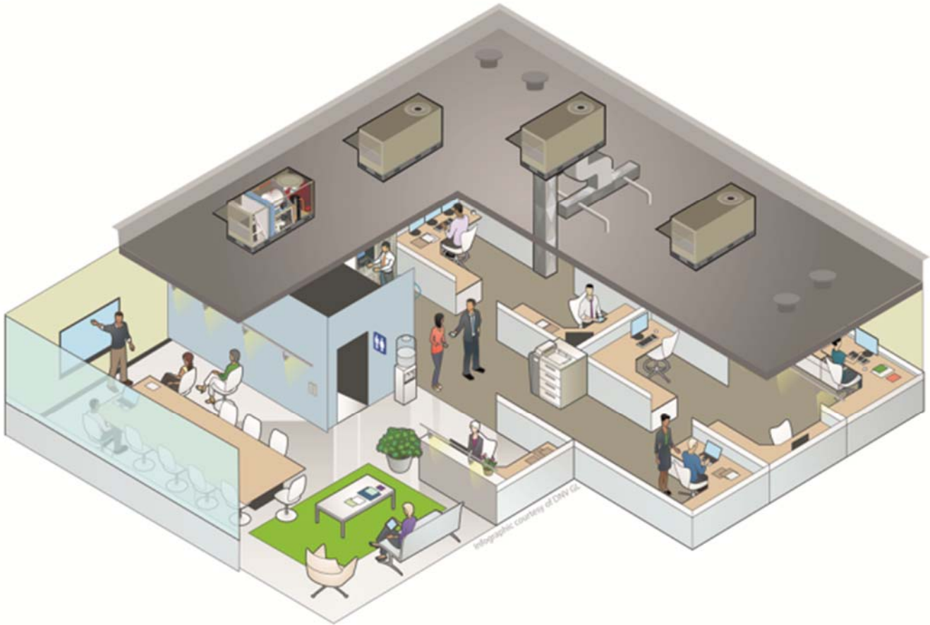
Figure 3. Installed packaged commercial air conditioner
