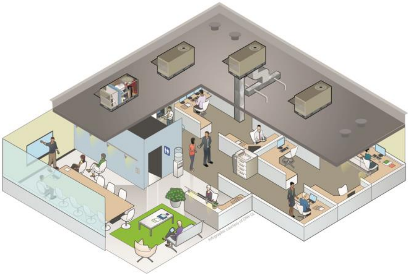
Figure 3. Installed packaged commercial air conditioner
