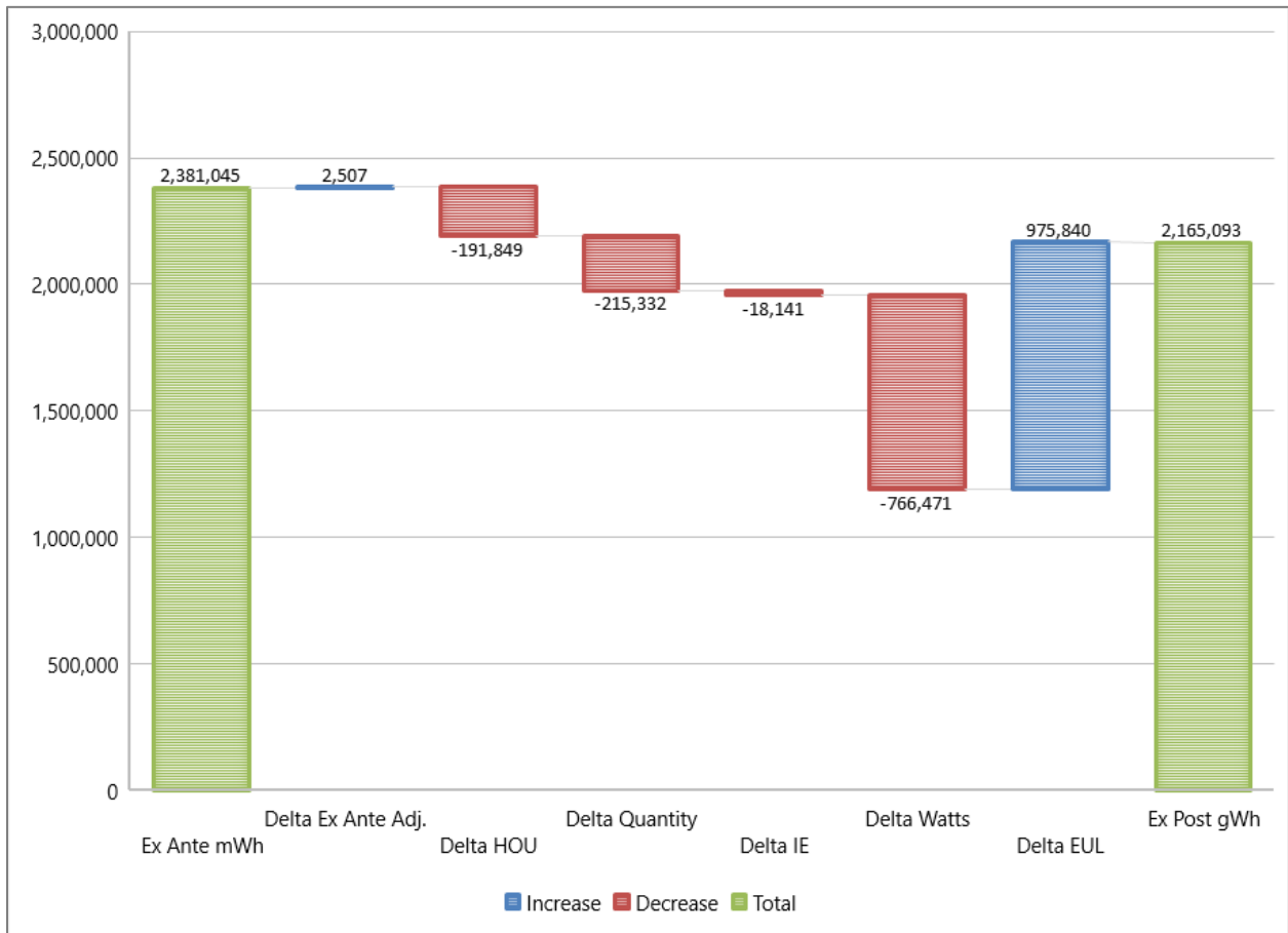
FIGURE 6-7: SDGE LED A-LAMP EX ANTE TO EX POST IMPACT WATERFALL
