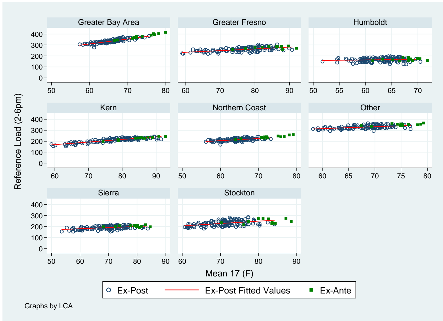
Figure 5-4: Comparison of Ex Post Reference Loads on Non-event Days to Ex-Ante Reference Loads for Large C&I
