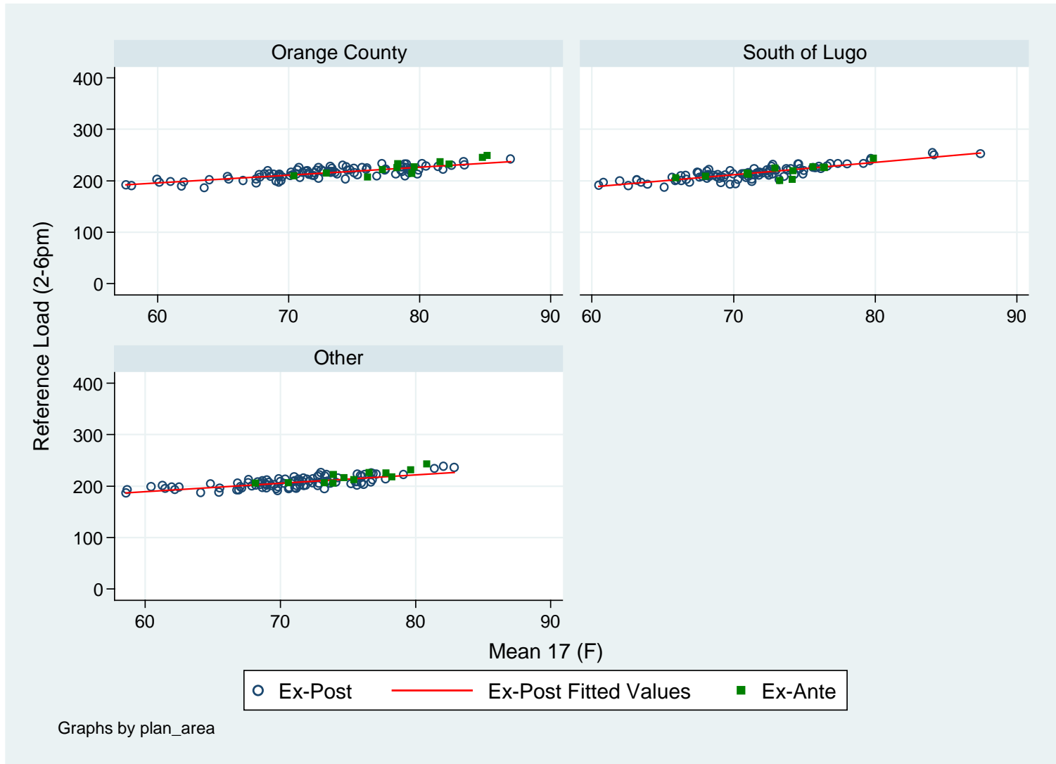
Figure 7-4: Comparison of Ex Post Loads on Non-event Days to Ex-Ante Reference Loads for Large C&I
