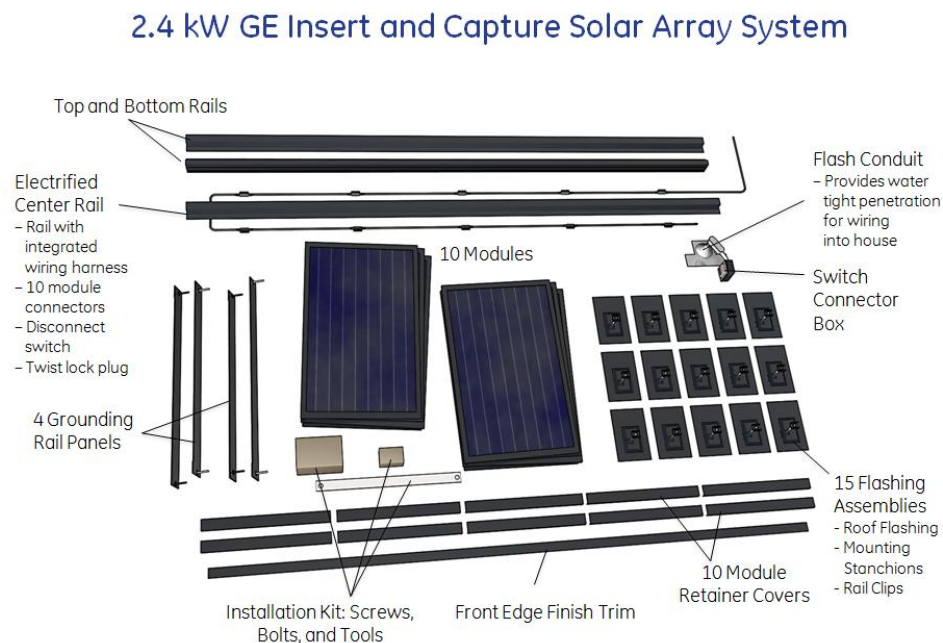
Figure 4: Illustration of the components of the Plug-and-Play VP Kit, illustrated here by the GE insert and capture 16-ft rail system.
