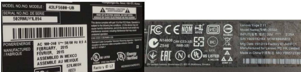
Figure 2. Labels Showing Manufacture Dates
